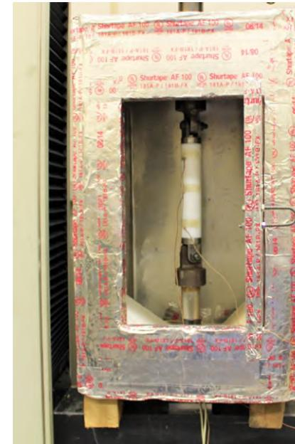
Entrance Bushing – vessel pressure boundary, transfers power from power supply to grid
