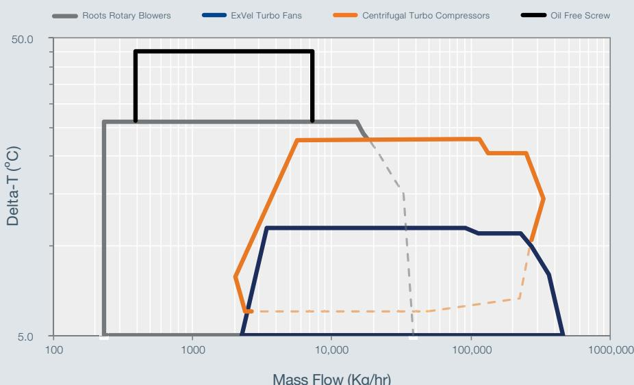
Chart depicts the potential performance from single stage equipment based on the properties of 100 °C (212 °F) saturated steam with 0.598 kg/m<sup>3</sup> density (0.0373 lb/ft<sup>3</sup>).
